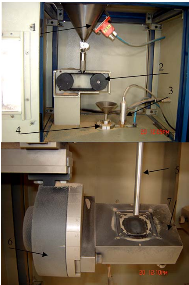
Fig. 1 Details of erosion test rig. (1) Sand hopper. (2) Conveyor belt system for sand flow. (3) Pressure transducer. (4) Particle-air mixing chamber. (5) Nozzle. (6) X–Y and \theta axes assembly. (7) Sample holder
